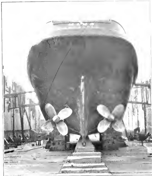
Stern view of the Mamo on dry-dock showing the clean run of the counter, large rudder, and solid bronze propellers.
